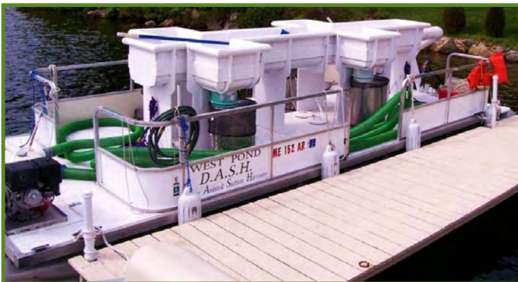
DASH units are constructed on floating platforms, such as a pontoon boat.
