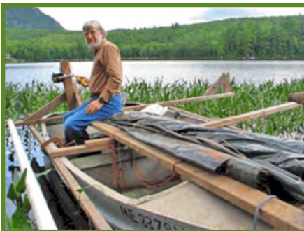
Jim Chandler with CLA's modified ATV winch mat-winder. This system, though somewhat finicky, was an improvement over the earlier bicycle crank-winder. Photo: Jim Chandler.
