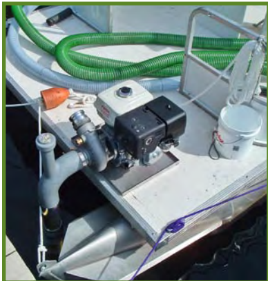
A venturi pump mounted on the deck of a DASH unit. Photo: Joe Howe.
